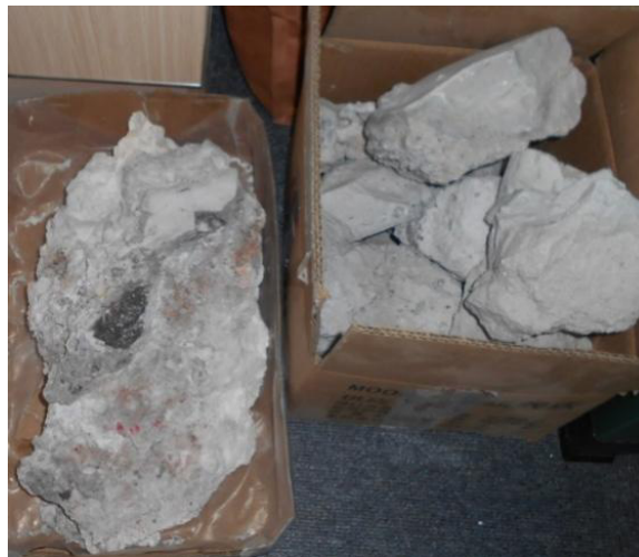
Figure 3. Solid cover removed from the butt of 200 kA cell.
