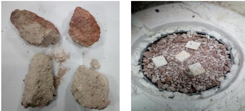
Figure 5. Solid covers removed from an anode butt of a 230 kA cell.
