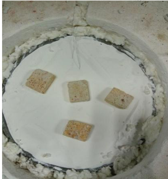
Figure 7. Alumina sample placed in heat conductor.
